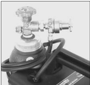
Figure 5 - Hose and Regulator Hookup
